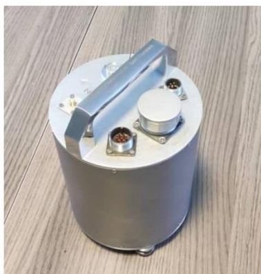
GP-PDS (GeoPersian Portable Digital Seismometer)
