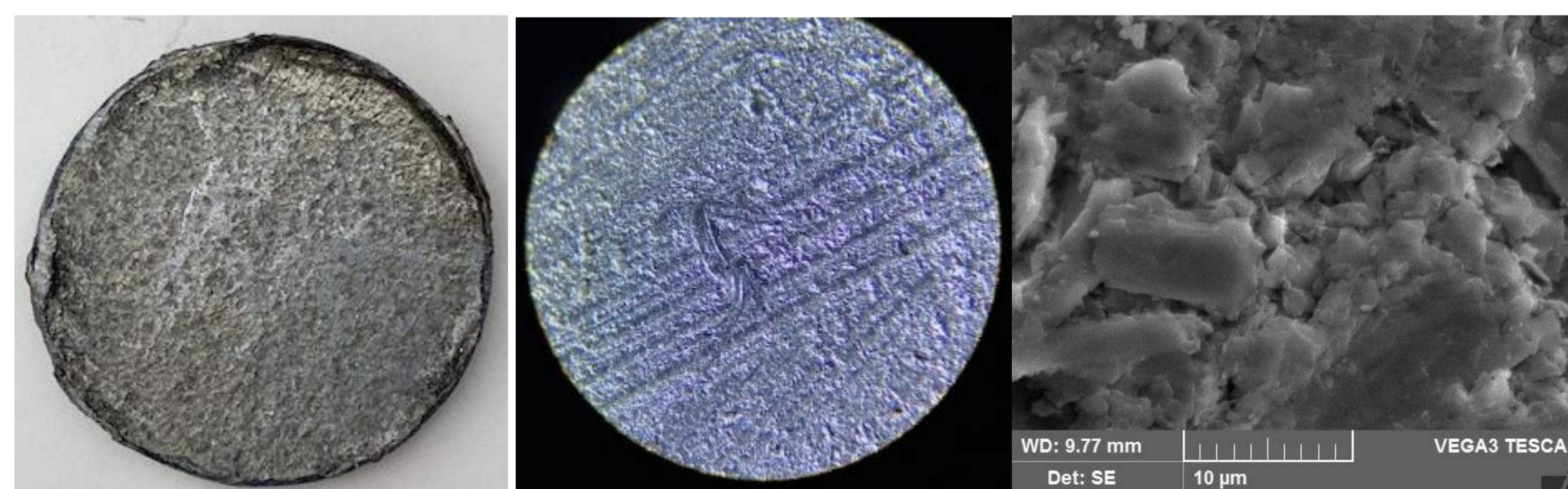
Figure 1) Optical, micrograph (X 10) & SEM (X 4K) images of Sintered sample
