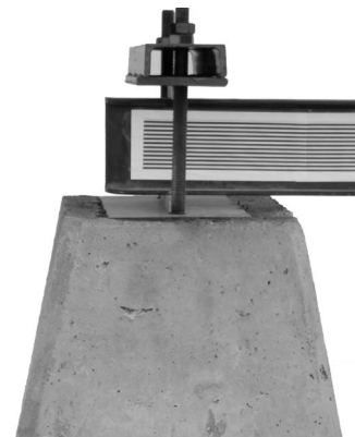
Fig. 4 Image of one end of the used I-beam on its massive base.
