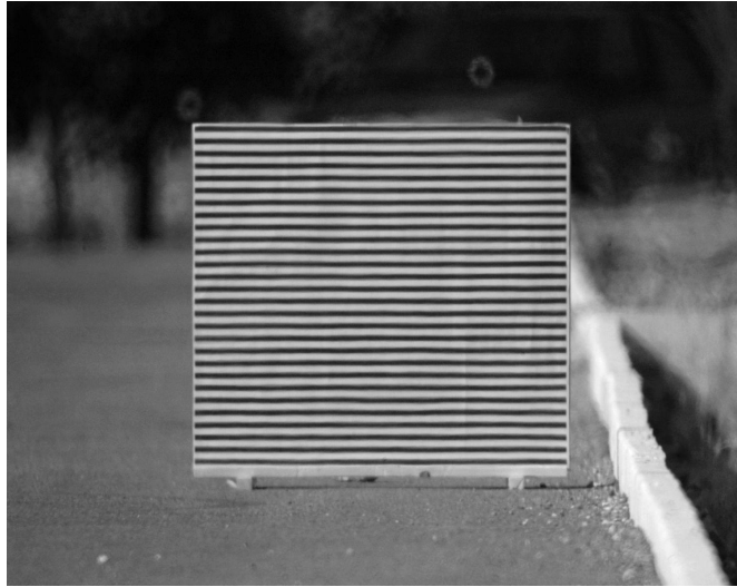
Figure 3. The image of the Ronchi grating with a pitch D=2.6\text{cm} , installed at the distance 89\text{m} from the imaging system. Exposure time was \frac{1}{250}\text{ses} . The fundamental angular frequency is 3.4\text{ Cycle/mrad} .
