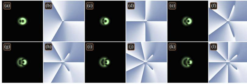
**Fig. 3.** Intensity (a,c,e,g,i,k) and phase (b,d,f,h,j,l) patterns of superposition (25) for the following parameters:  $\lambda = 532$  nm,  $w = 500$   $\mu$ m,  $m = 2$ ,  $n = 3$  (a,b),  $n = 4$  (c,d),  $n = 5$  (e,f),  $n = 6$  (g,h),  $n = 7$  (i,j),  $n = 8$  (k,l),  $A = B = 1$ ,  $x_0/w = 0.5$  (a-l). Computing area  $|x|, |y| \leq R$  ( $R = 5$  mm).
