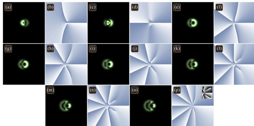
**Fig. 4.** Intensity (a,c,e,g,i,k,m) and phase (b,d,f,h,j,l,n) patterns for superposition (25) at  $\lambda = 532$  nm,  $w = 500$   $\mu$ m,  $n = 1$  (a,b), 2 (c,d), 5 (e,f), 6 (g,h), 7 (i,j), 8 (k,l), 9 (m,n), 10 (o,p),  $A = B = 1$ ,  $x_0/w = 0.5$ . Computing domain  $|x|, |y| \leq R$  [ $R = 5$  mm (a-o) and  $R = 50$  mm (p)].
