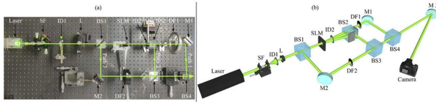
**Fig. 7.** Used experimental setup (a), and the corresponding schematic arrangement (b). SF, ID, L, BS, SLM, DF, and M show spatial filter, iris diaphragm, lens, beam splitter, density filter, and mirror, respectively.
